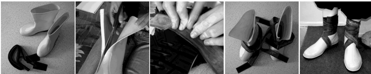
Figure 1. step-by-step images on re-forming boots.
